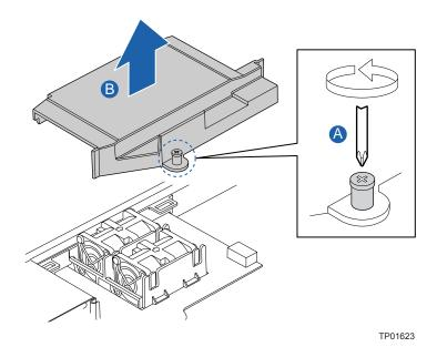
Figure 41. Removing the Power Supply Air Duct
